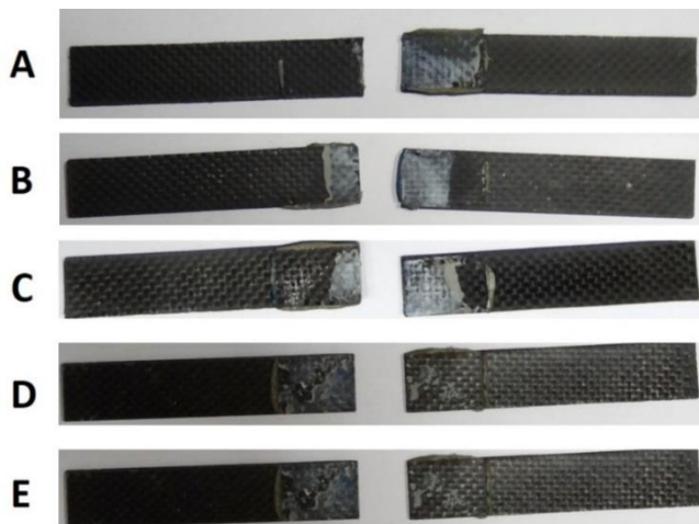
Figure 2. Fracture diagram of samples connected by different adhesives, (A) Loctite 406 instant adhesive, (B) Loctite 496 instant adhesive, (C) DP-460 epoxy resin adhesive, (D) M1-05 acrylic adhesive and (E) MAXLOKT6 acrylic adhesive.
